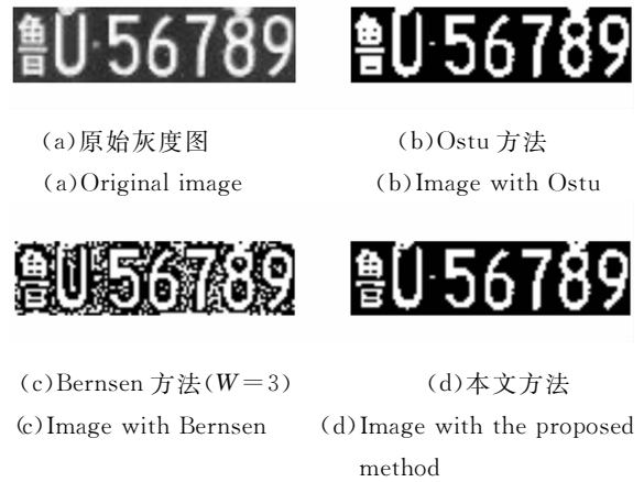
图 3 车牌号码正常拍摄时三种方法比较 Fig. 3 Three methods comparison under normal photography for vehicle license plate
