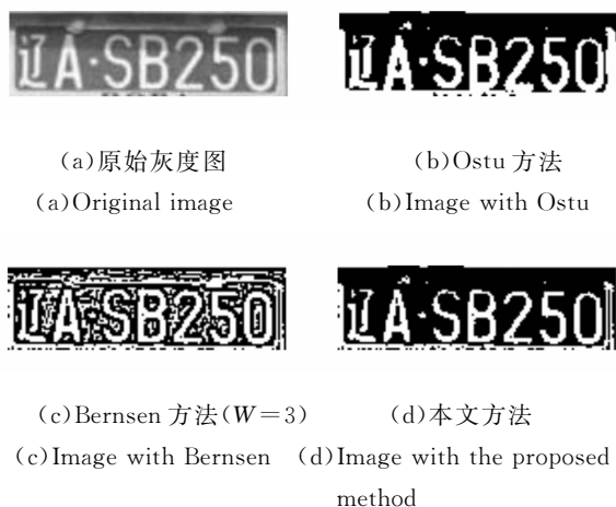
图5 车牌号码上方有阴影时三种方法比较 Fig. 5 Three methods comparison under shadow photography for vehicle license plate
